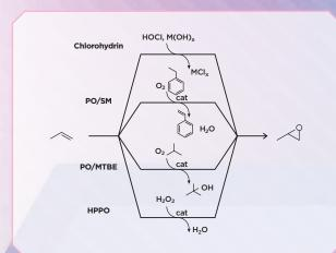
There are several technologies of propylene epoxidation with hydrogen peroxide using methanol as a propylene solvent. Techinservice uses acetonitrile as a propylene solvent, which drastically reduces the amount of process byproducts.
