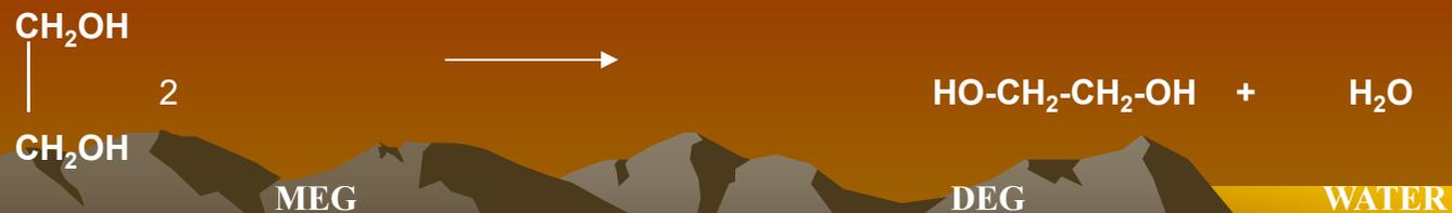
The DEG content in the final product can therefore be controlled within certain limits by corresponding process alterations. The DEG molecules are built instead of MEG molecules in the polymer chain.
