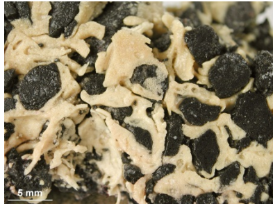
Figure 5. Doughy texture - OMR-binder has a character of dough pushed into gaps between the conglomerate grains, it does not fill fully the voids and does not stick fully to the grains.
