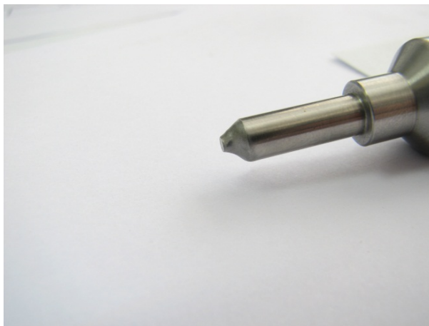
Figure 10. Mixing head needle corrosion by EG
