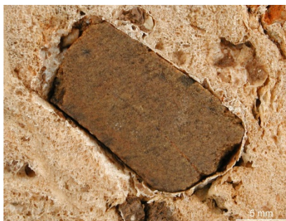
Figure 4. Honeycomb texture III. (free rock particle can be taken out of the PUR-binder „tissue”).
