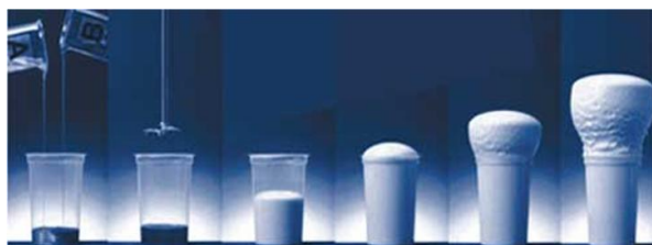
Figure 2. Polymerization of the palm-based polyurethane
