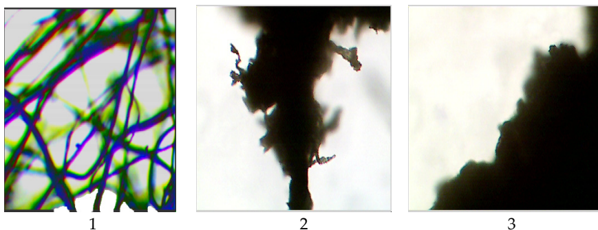
1 – initial polysaccharide fibers; 2 - effect of aggressive microbial medium; 3 – effect of natural microbial medium.
