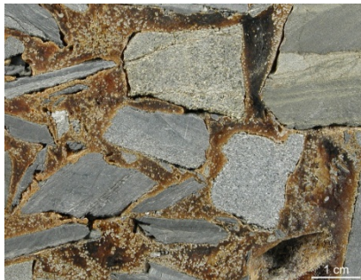
Figure 3. Honeycomb texture II. (PUR is surrounding the rock particles, but sticks only partly to their surface).
